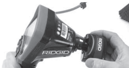
Figur 19 – Kameraets tilkopplingsplugg installert
